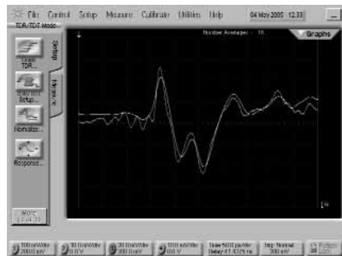
Figure 4: Corrected impedance profile (green trace)
