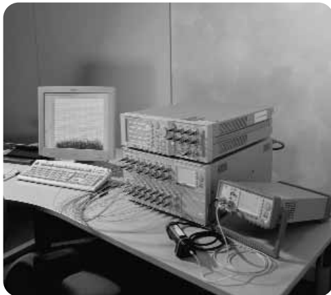
40ch spectrum analysis synchronizing tunable laser source and power meter
